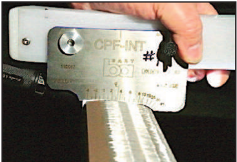
Template used in rail grinding which provides the specified shape the rail should be ground to. It represents what the final profile should look like.
